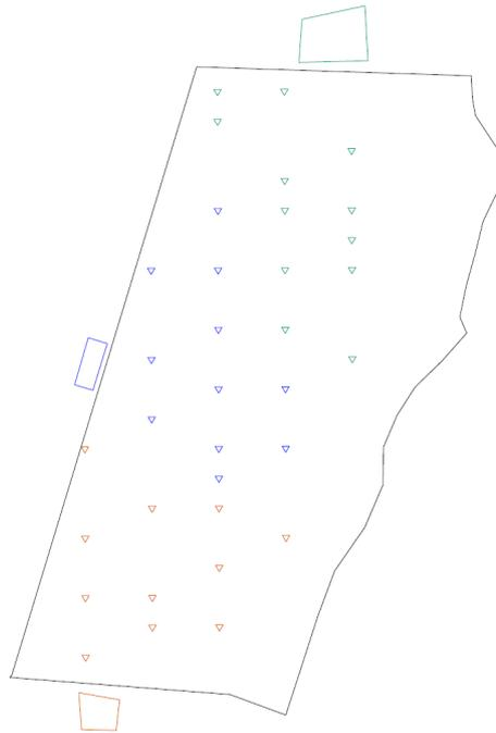
Figure 8.1: Schematic view of a case with a single available area and three first level interconnection facilities when applying balanced distribution. Triangles are power stations, and they are in the same color as the facility to which they have been assigned.
