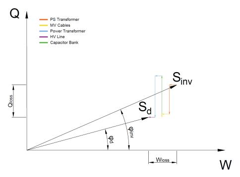
Figure 5: Phasor representation of the phi angle at the delivery point with capacitor banks compensating the power transformer
