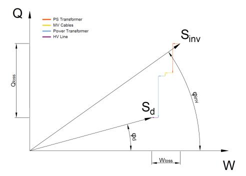
Figure 2: Phasor representation of the phi angle at the delivery point (not to scale)
