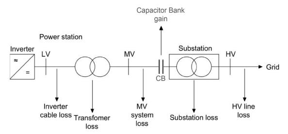
Figure 3: Diagram of the AC transmission system model with capacitor bank
