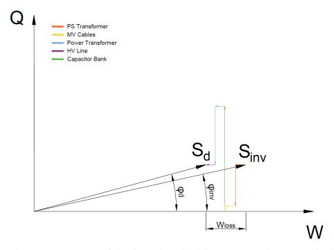
Figure 4: Phasor representation of the phi angle at the delivery point with capacitor banks compensating all the systems
