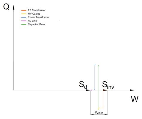
Figure 6: Phasor representation of the phi angle at the delivery point with capacitor banks compensating the all the systems with a required power factor of 1
