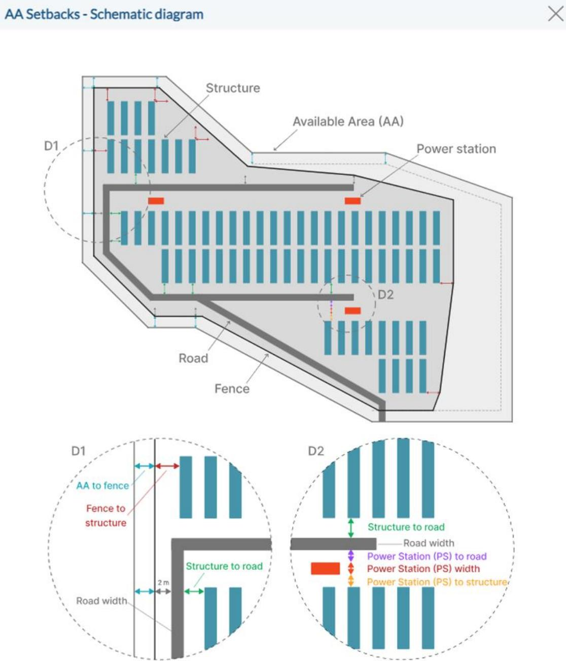
Figure 5.4.6.2. Schematic diagram for AA setbacks.
