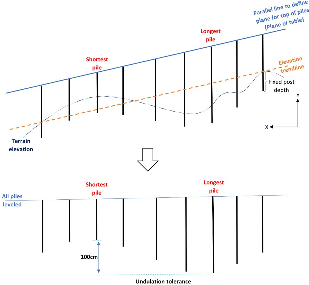
Figure 5.5.1.9. Visual representation of how the undulation tolerance limit works.
