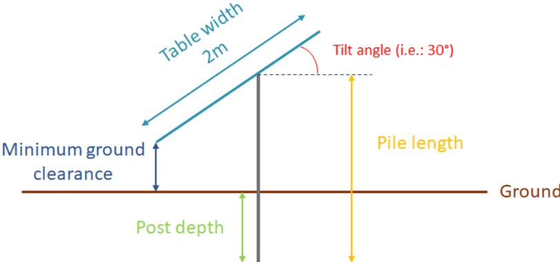
$$\text{Pile Length} = \text{Post Depth} + \text{Minimum Ground Clearance} + (\text{Table width} \cdot 2/3) \cdot \sin(\text{Tilt angle})$$
