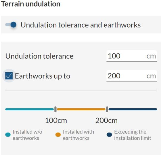
Figure 5.5.1.8. RatedPower's analysis tool for undulation tolerance criterion.
