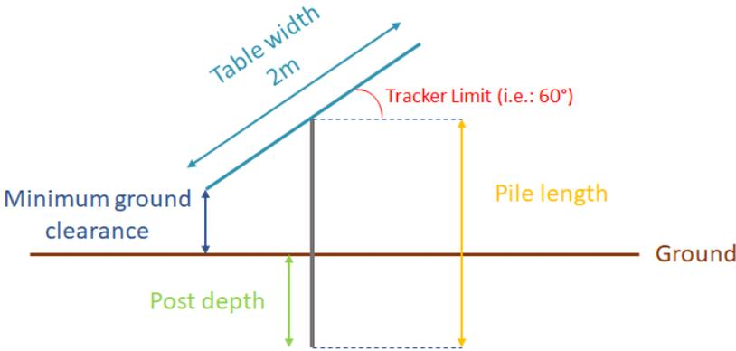
$$\text{Pile Length} = \text{Post Depth} + \text{Minimum Ground Clearance} + (\text{Table width}/2) * \sin(\text{Tracker Limit})$$
