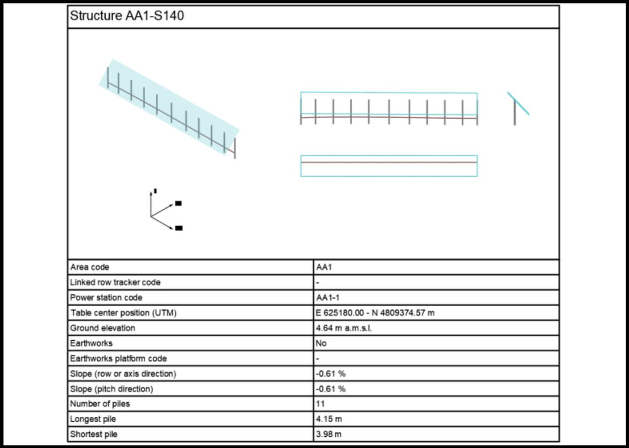
Figure 8.3.8. Example of the structure profiles CAD file.
