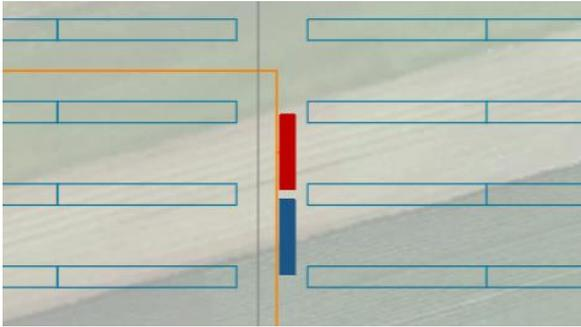
Figure 5.8.2. DC-BESS containers in the layout.
