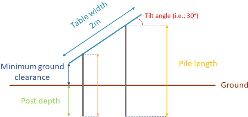
$$\text{Pile Length} = \text{Post Depth} + \text{Minimum Ground Clearance} + (\text{Table width} \cdot 3/4) \cdot \sin(\text{Tilt angle})$$
