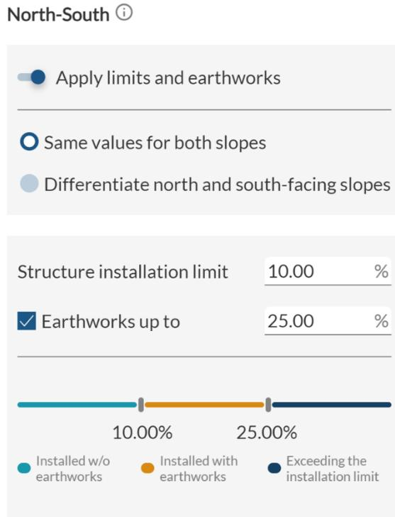
Figure 5.5.2. RatedPower's earthwork tool example.
