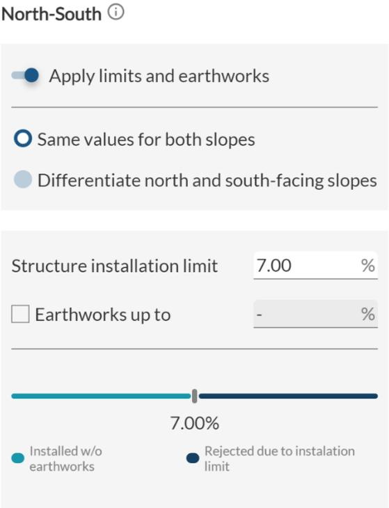
Figure 5.5.1.5. RatedPower's topography analysis tool for North-South criteria
