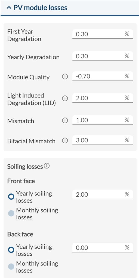
Figure 5.9.4. PV modules losses.
