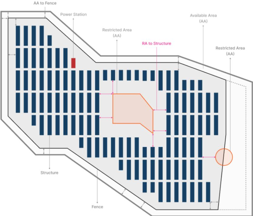
Figure 5.4.6.6. Schematic diagram for RA setbacks.
