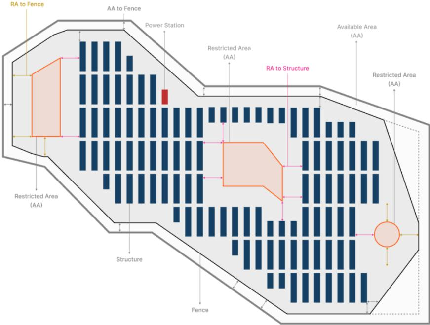
Figure 5.4.6.5. Schematic diagram for RA setbacks.
