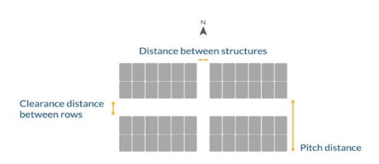
Figure 5.4.3.2. Pitch distance and distance between consecutive structures in fixed structures.
