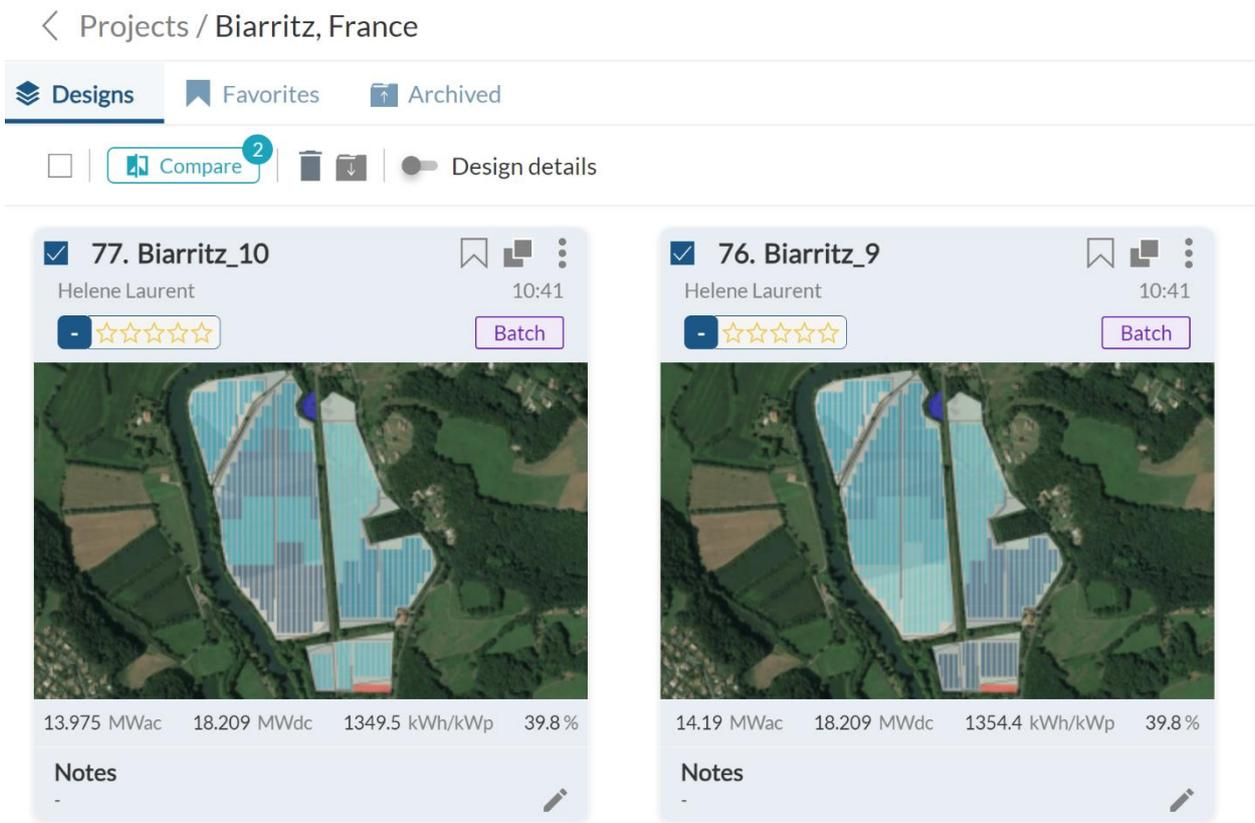
Figure 4.5. RatedPower's comparison tool.
