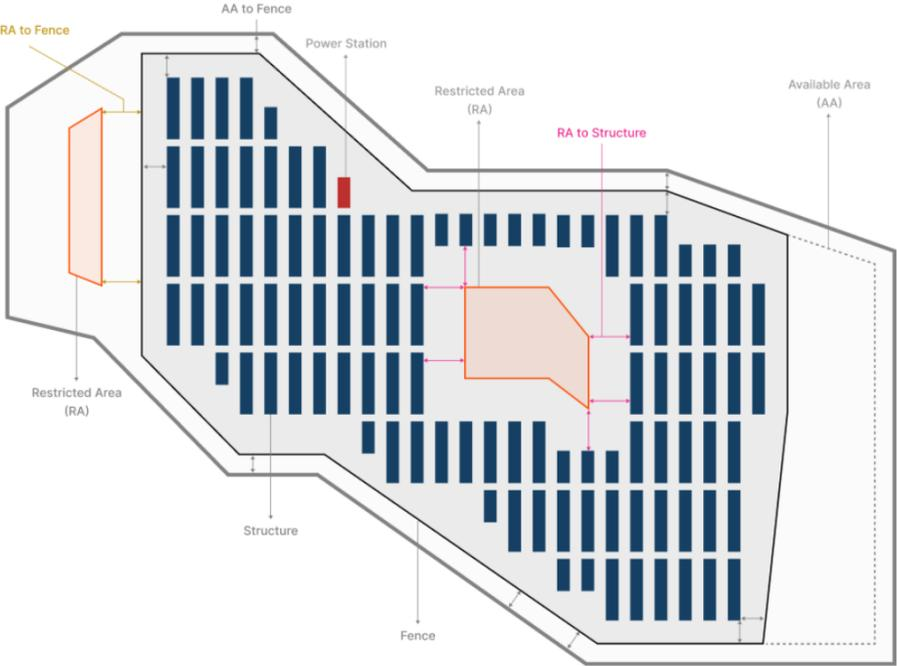
Figure 5.4.6.4. Schematic diagram for RA setbacks.
