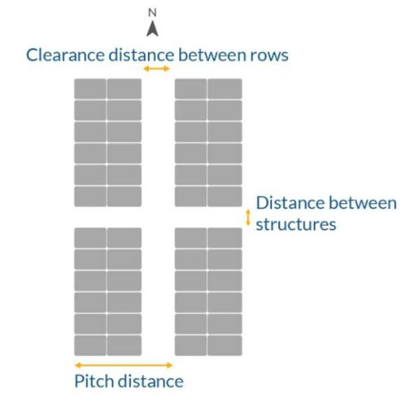
Figure 5.4.3.3. Pitch distance and distance between consecutive structures in trackers
