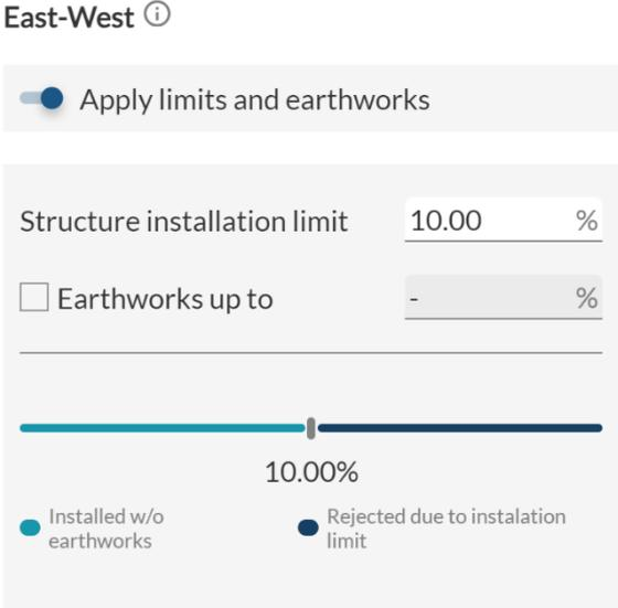
Figure 5.5.1.7. RatedPower's topography analysis tool for East-West criteria.
