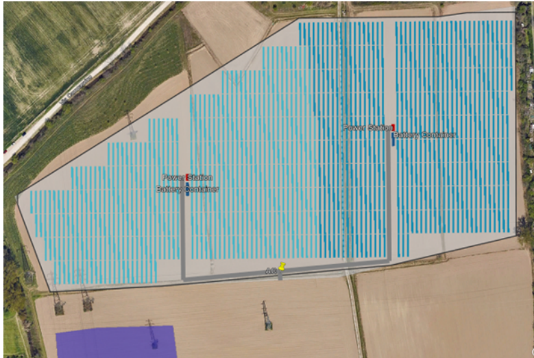
Figure 3.1: The battery containers are connected to all the power stations. Source: RatedPower
