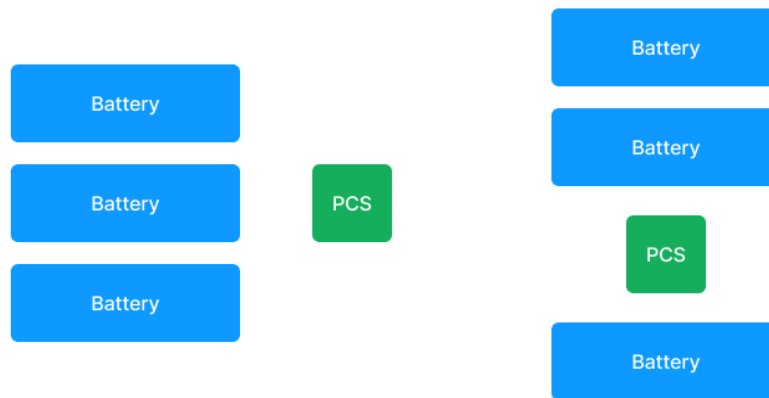
Figure 2.4: PCs in front at the left. PCS in side at the right. Source: RatedPower
