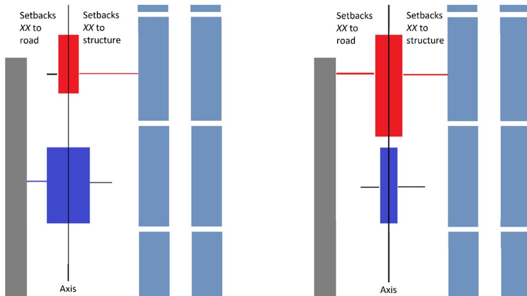
Figure 3.4: Distances between containers and roads or structures. Source: RatedPower
