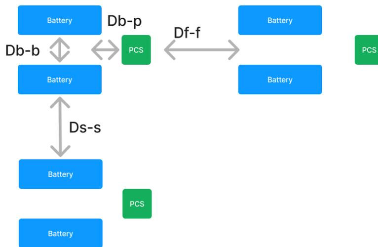
Figure 2.2: Safety distances between battery power blocks. Source: RatedPower
