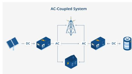
Figure 1.1: AC-coupled battery energy storage system diagram. Source: RatedPower
